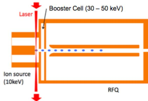
Figure 4: A conceptual image of the accelerator front end with the short pulse laser ion source.
