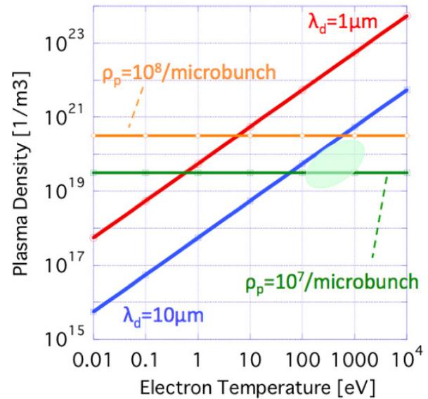
Figure 1: Condition of short pulse ion beam production. The region colored by light green is suitable for the production of short pulse ion beam.
