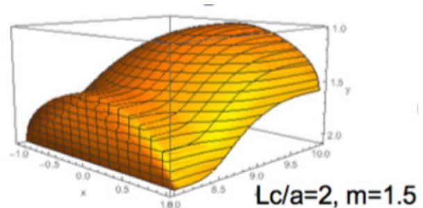
Figure 5: A trapezoidal vane shape for high efficiency acceleration.
