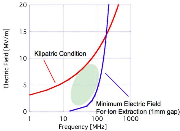
Figure 2: The relation between amplitude and frequency of the extraction electric field. The region colored by light green is suitable for the extraction of the ions
