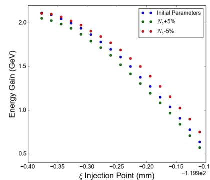
Figure 4: Energy gain of injected electrons for  $z > 4$  m as a function of  $\xi$  in the optimal region for initial and  $N_b \pm 5\%$  runs (injection  $-12.03 < \xi < -11.99$  cm).
