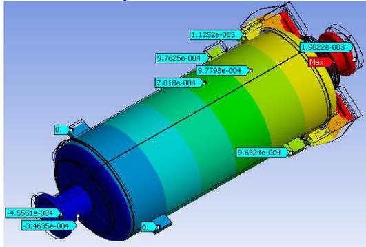
Figure 6: Cavity displacements due to cool-down to 2K.
