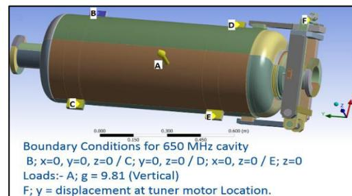
Figure 4: Loads and boundary conditions for simulations
