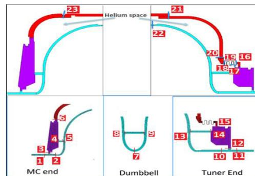
Figure 5: Stress classification lines on dressed cavity
