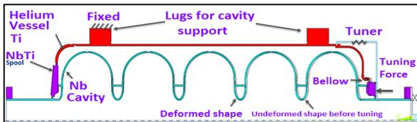
Figure 3: 2D axis-symmetric dressed cavity model.
