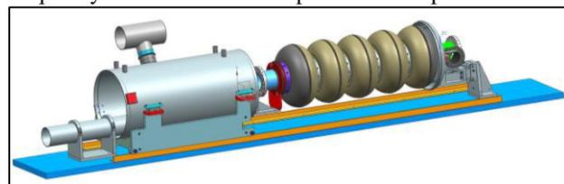
Figure 9: Insertion device for cavity dressing.
