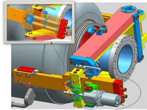
Figure 8: Double Lever tuner mechanism for 650 cavity.
