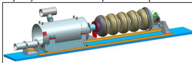
Figure 9: Insertion device for cavity dressing.
