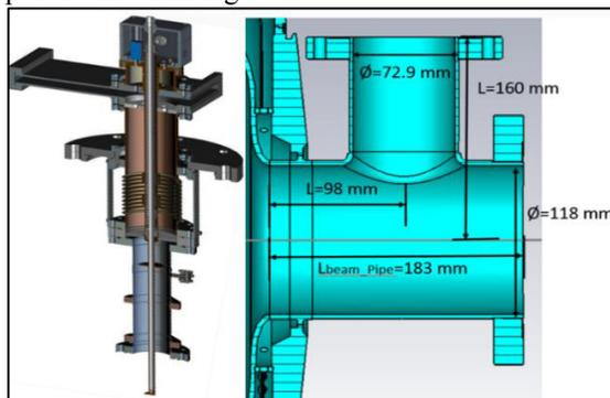
Figure 7: 650 MHz coupler and ports for LB650 and HB650 cavities.
