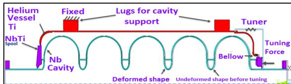
Figure 3: 2D axis-symmetric dressed cavity model.
