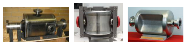
Figure 19: Proof-of-principle cavities: 4-rod cavity (left), double quarter wave cavity (middle), and rf-dipole cavity (right).
