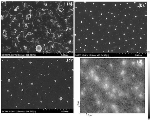
Figure 2: SEM images of samples with a nucleation time of one hour at various nucleation temperatures: (a) 400 °C, (b) 450 °C, (c) 500 °C. EDS was only able to identify tin from bright circular features. SAM elemental mapping of tin coverage from the sample treated at 500 °C for one hour is shown in (d). Note that surface produced after one hour at 400 °C appears very different.
