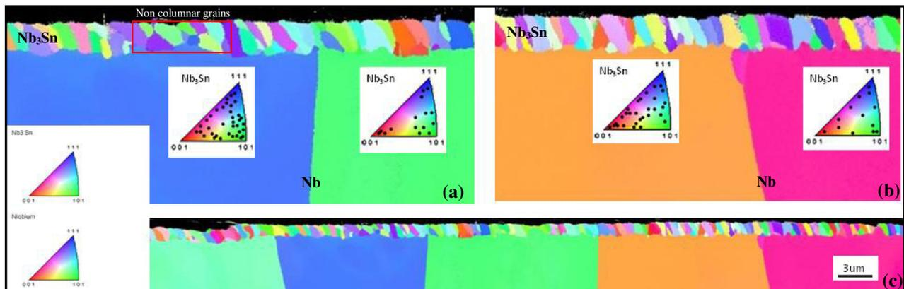
Figure 6: EBSD image of the cross-section from sample U3 is shown in (c). Smaller grains on the top are Nb<sub>3</sub>Sn. Larger grains at the bottom are Nb. Images (a) and (b) are magnified areas from (c). Approximate orientations of Nb<sub>3</sub>Sn grains on each Nb grain are shown with inverse pole figure using assigned color for each grain. Each dot represents an individual Nb<sub>3</sub>Sn grain.
