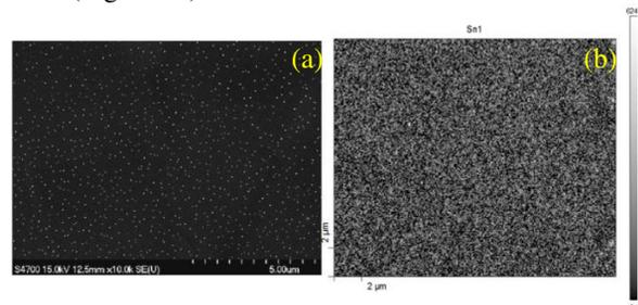
Figure 4: (a) SEM image of nucleated surface obtained by using Cornell recipe. (b) SAM elemental mapping of tin.
