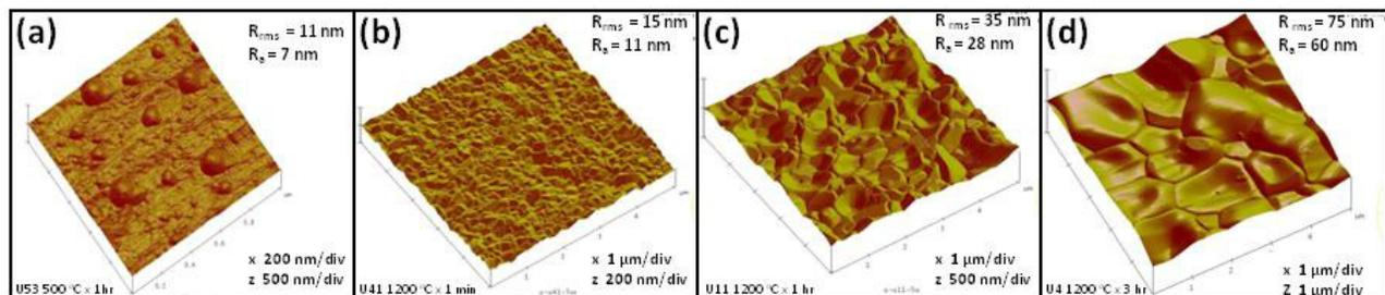
Figure 5: AFM images shows grain growth and topography evolution during the coating process. (a) Sample treated at 500 °C for one hour. The scan size is 1 μm x 1 μm. (b) Sample treated at 1200 °C for one minute, (c) 1200 °C for one hour and (d) 1200 °C for three hours. The scan size for images (b) – (d) is 5 μm x 5 μm.
