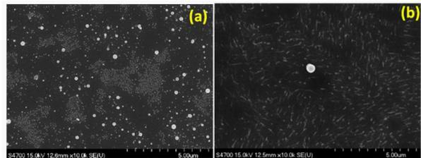
Figure 3: SEM images of samples obtained from experiments with a nucleation temperature of 500 °C and nucleation time of (a) 4 hours and (b) 5 minutes.
