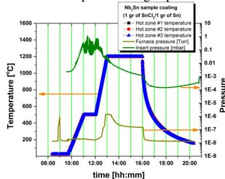
Figure 1: Temperature profile used for coating Nb<sub>3</sub>Sn onto niobium samples. The nucleation process occurs at the first temperature plateau of 500 °C and deposition proceeds at the 1200 °C temperature plateau.
