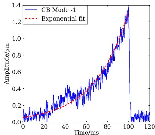
Figure 5: Amplitude of the -1 coupled-bunch mode with the bunch-by-bunch feedback turned off for the first 100 ms and then turned on again.
