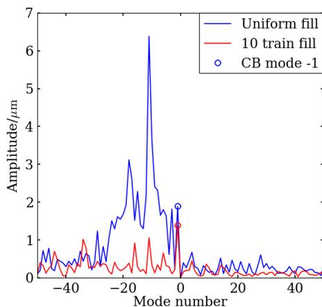
Figure 4: Coupled-bunch mode spectra for two filling patterns: a uniform fill of 47 mA and 52 mA in a fill of ten bunch trains with gaps between them of 3, 10 or 11 bunches.
