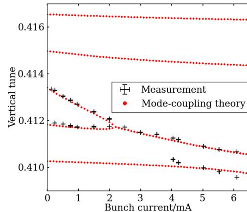
Figure 3: Peak frequencies as measured using an excitation around the betatron frequency for different bunch currents at a vertical chromaticity of 0.7.
