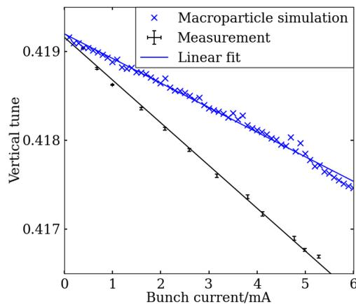
Figure 2: Tune as measured using the bunch-by-bunch feedback system as a function of single bunch current at low chromaticity.
