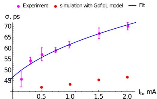
Figure 1: Bunch length vs. current: measurements in magenta (set of five measurements), simulations with *mbtrack* with full numerical machine impedance in red and fit including a single broadband resonator in blue.
