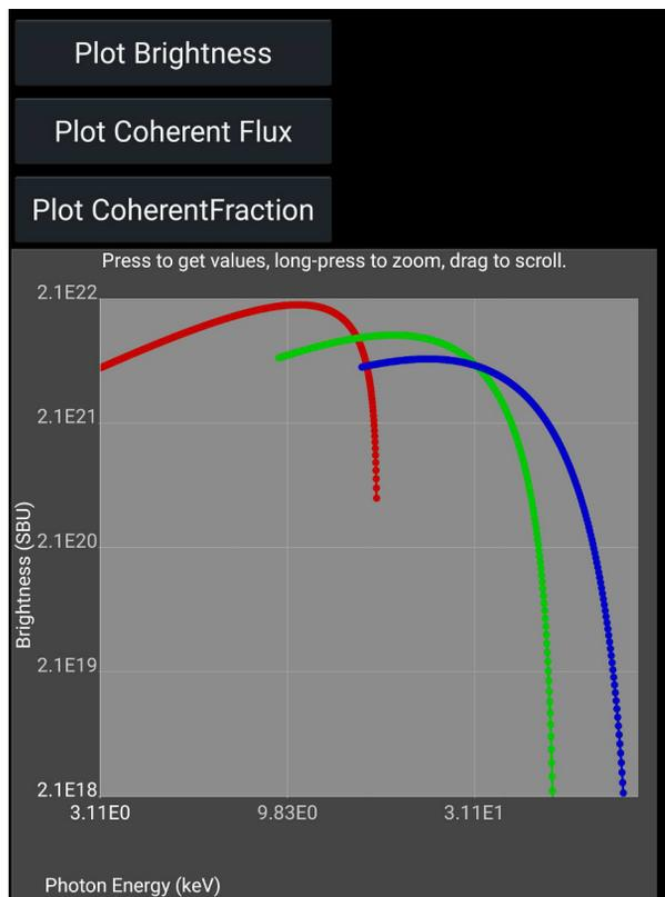
Figure 5: Example of undulator brightness curves for the 67-pm APS upgrade lattice with a 20-mm-period SCU.
