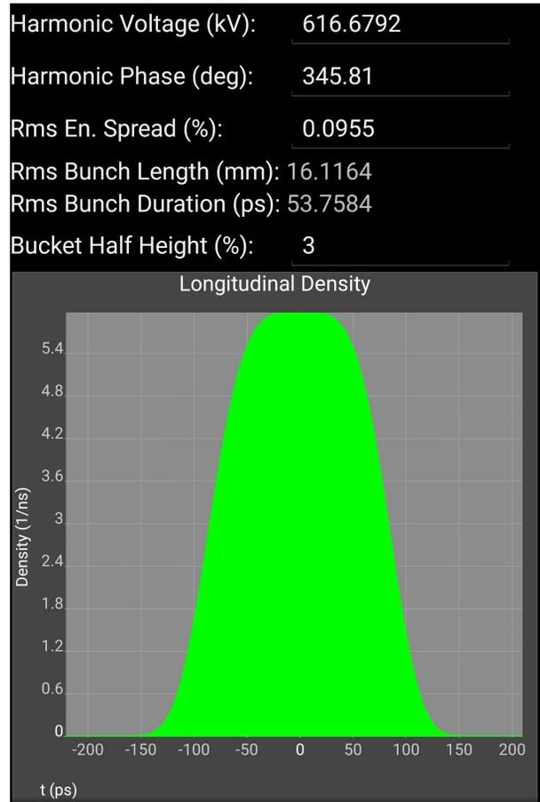
Figure 3: Example of optimization of a 4th-harmonic bunch lengthening cavity for the APS upgrade.
