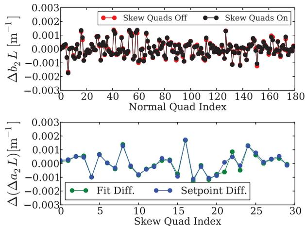
Figure 2: DTBLOC estimates of focusing ( $\Delta b_2 L$ ) and skew quadrupole ( $\Delta a_2 L$ ) errors for the 2 different cases “skew on” and “skew off”.
