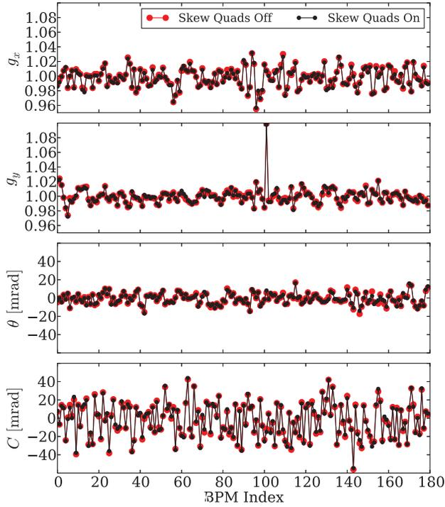
Figure 1: DTBLOC estimates of BPM errors for the 2 different cases “skew on” and “skew off”.
