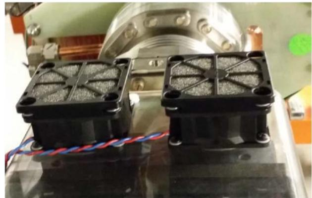
Figure 6: Cooling fans installed on the safety plastic shielding of each kicker pulse magnet.
