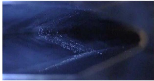
Figure 4: Kicker 2 chamber internal view after de-installation from the storage ring. O-Ring damaged shape of Ti-coating observed at the upstream of the chamber.
