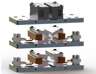
Figure 3: Top: Blank Magnet Module prior to EDM; Middle: Magnet Module 1 post EDM, plating, and assembly; Bottom: Magnet Module 9 post EDM, plating, and assembly.
