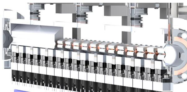
Figure 2: Array of magnets from the a bifurcated view of the insert. Portions of the vacuum chamber are hidden.
