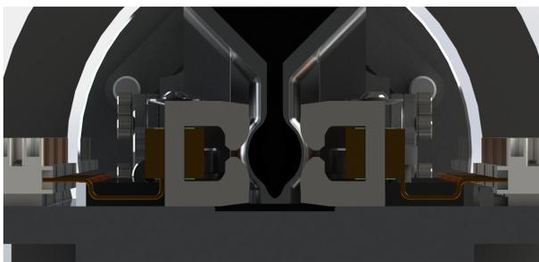
Figure 5: View of the vacuum chamber inside of a magnet module.
