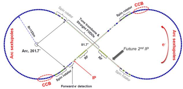
Figure 1: Top view layout of the electron ring.
