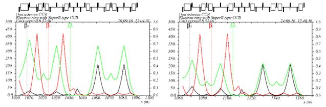
Figure 6: Optics of low emittance CCB schemes 4 and 6.
