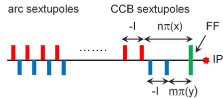
Figure 3: Schematic of two non-interleaved  $-I$  sextupole pairs on one side of IP.
