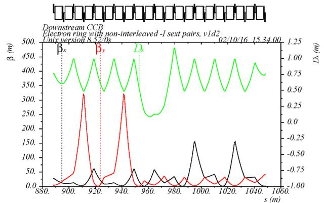
Figure 4: CCB optics with two non-interleaved  $-I$  sextupole pairs based on arc cell configuration.
