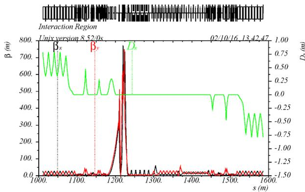
Figure 2: Optics of the electron ring long straight section with the IP before including FF chromaticity correction.
