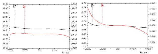
Figure 8: Tune (left) and  $\beta^*$  (right) versus  $\Delta p/p$  with low emittance CCB scheme-6.
