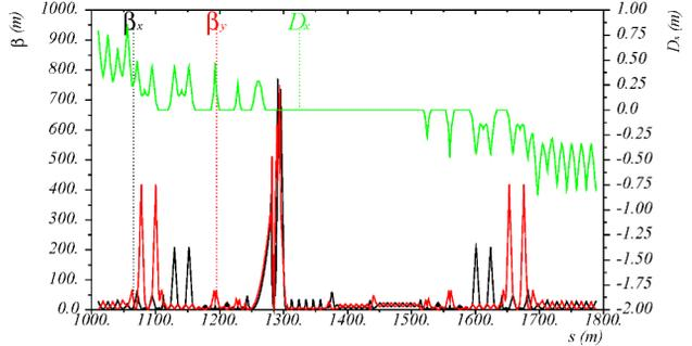
Figure 7: Straight section with the IP and low emittance CCB based on scheme-6.
