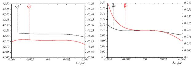
Figure 5: Tune (left) and  $\beta^*$  (right) versus  $\Delta p/p$  with CCB based on arc cells and non-interleaved  $-I$  sextupole pairs.
