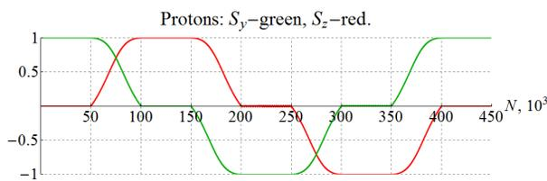
Figure 6: Rotating the proton spin in an ideal collider lattice.
