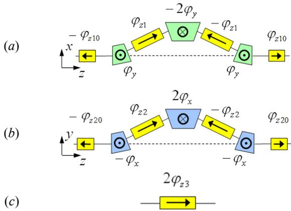
Figure 2: Modules for control of the radial (a), vertical (b), and longitudinal (c) spin components.
