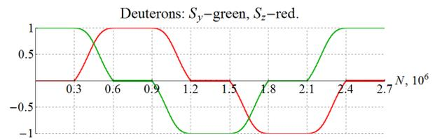
Figure 8: Rotating the deuteron spin in an ideal collider lattice with the adiabatic condition of the spin motion satisfied.
