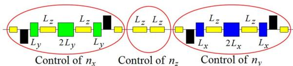
Figure 3: Placement of the 3D spin rotator elements.
