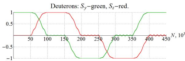
Figure 7: Rotating the deuteron spin in an ideal collider lattice with violation of the adiabaticity condition of the spin motion.
