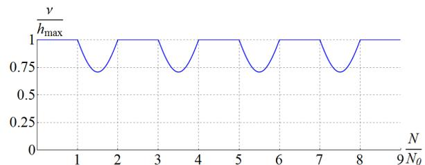
Figure 5: Change in the spin tune in units of the maximum spin field  $h_{max}$  when rotating the spin in the collider.
