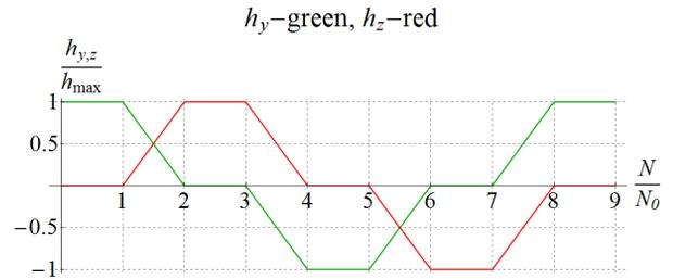
Figure 4: Pattern of change in the vertical  $h_y$  and longitudinal  $h_z$  spin field components when making spin reversals in the collider ring.
