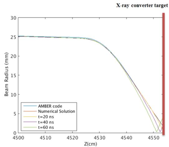
Figure 6: The time varying beam radius on a target with back streaming ions (protons).
