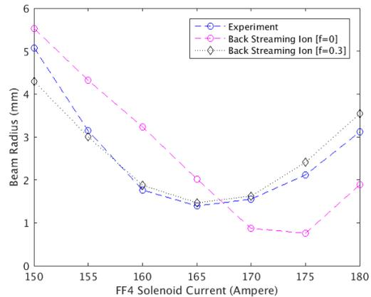
Figure 7: Comparison of x-ray spot size data with spot size form numerical solution, both have good agreement when neutralization factor  $f=0.3$ .
