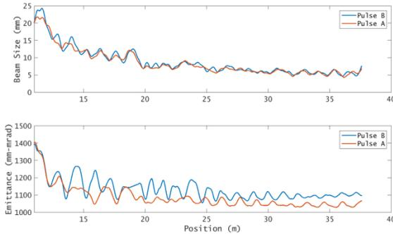
Figure 4: The rms beam envelope and Lapostolle normalized emittance from the accelerator entrance to the diagnostic cross, with an optimized magnetic tune for two electron pulses with different acceleration scheme.
