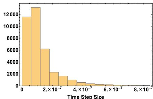
Figure 7: Time step sizes histogram of the whole run for relativistic protons when bins are of equal number of particles.
