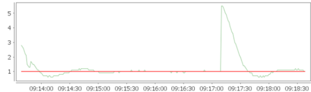
Figure 5: Phase vs. clock time for the process variable in green and the set point in red.
