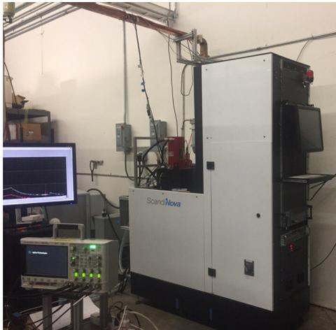
Figure 3: Klystron's collector visible from the modulator mounting and the high power isolator from Ferrite Inc. mounted to the wall directly behind it.
