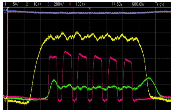
Figure 7: Oscillogram of six beam pulses injected into a single 5  $\mu$ s RF pulse. Yellow is the incident RF power (nominally 5 MW), green is the power transmitted to the load on the output coupler of the linac, and pink is the current accelerated and detected by a self-integrating current transformer.
