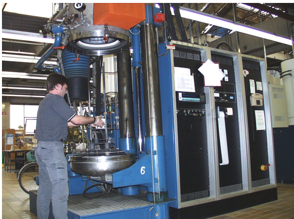
Figure 2: Vacuum braze furnace being loaded with an insulator.
