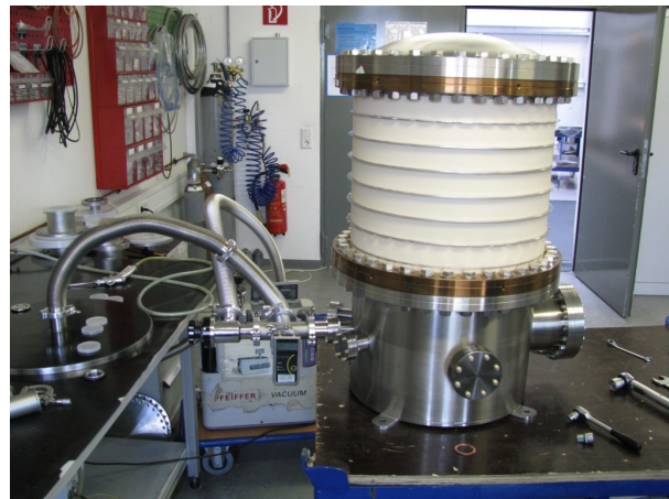
Figure 5: Insulator factory acceptance testing.
