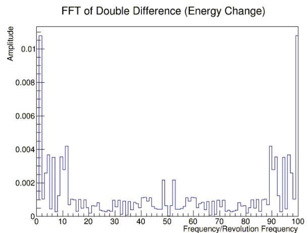
Figure 3: FFT of difference in electron and positron orbit differences due to sinusoidal energy change of amplitude one part in  $10^4$ .
