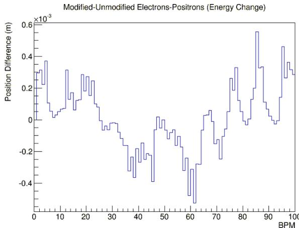
Figure 1: Difference in electron and positron orbit changes when changing energy sinusoidally around the ring with amplitude one part in  $10^4$ .
