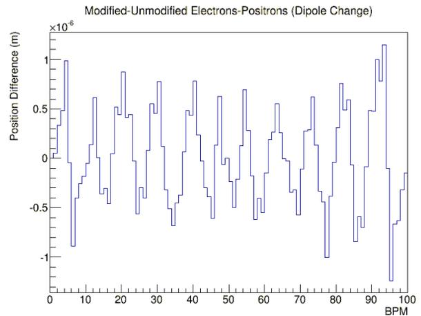
Figure 2: Difference in electron and positron orbit changes when changing dipole strength by one part in  $10^4$ .
