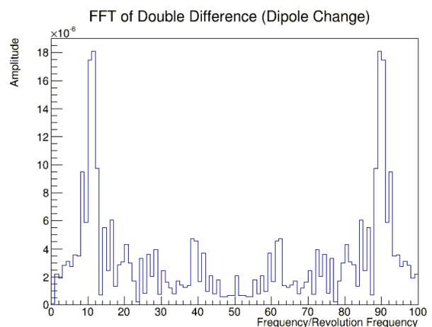
Figure 4: FFT of difference in electron and positron orbit differences due to dipole strength change of one part in  $10^4$ .
