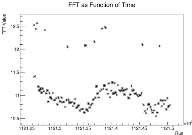
Figure 5: Plot of FFT value at the revolution frequency for difference between electron and positron orbits as a function of time. We are clearly able to pick out the time when we had the RF cavity voltages shifted to a different value (runs 112136 - 112145). However, there is a similar change at the start of data-taking, when we were not doing anything, which would dramatically reduce our sensitivity if we do not have it under control.
