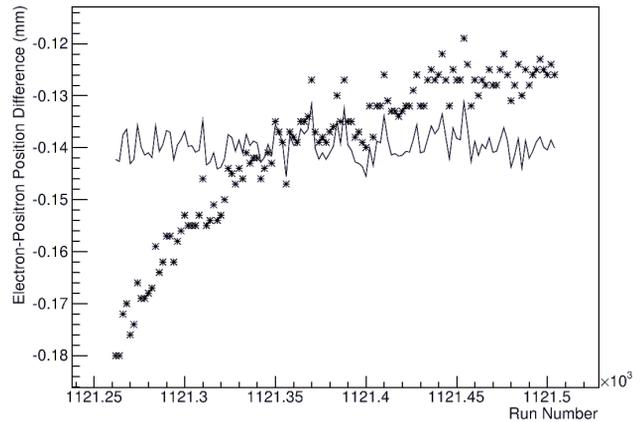
Figure 6: Electron/positron orbit difference at BPM 17 as a function of time. The points show the measured data, while the line shows the resulting orbit difference if one corrects for a hypothetical current-dependent gain. We see that such a current-dependent gain would explain our measured orbit change.
