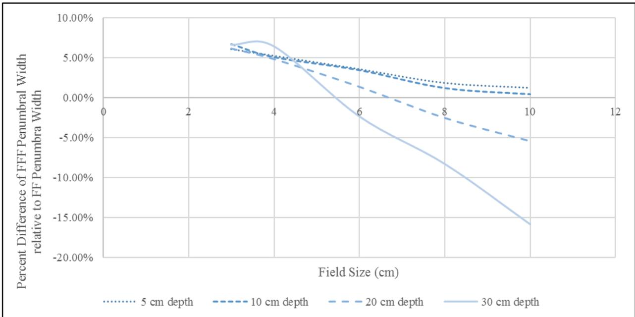
Figure 1 (top): Percent difference in dose relative to central axis between FFF beams and FF beams. Negative values indicate that relative dose for the FFF beam was lower than relative dose for the FF beam at the same location.
