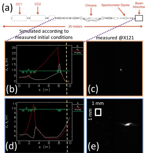
Figure 3: Overview of the interfacing of FAST injector beamline (a) and corresponding evolution of the betatron function before (b) and after (d) beam matching to achieve a small beam size at the location of X121. Image (c) and (e) are the corresponding measured beam density at X121.
