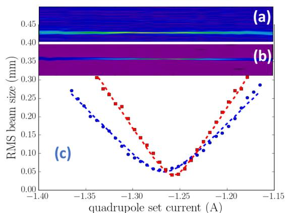
Figure 2: An example of quadrupole scan. Insets (a) and (b) show a 2-D image of the stack horizontal (a) and vertical (b) profiles. The associated rms beam sizes (in this example obtained from Gaussian fits of the profiles) are shown in (c).
