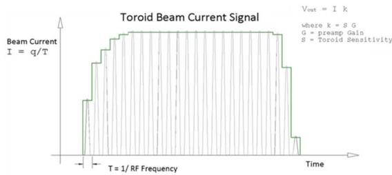
Figure 3: Processing the envelope of the toroid's beam current signal.
