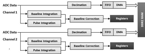
Figure 6: Simplified data path for the digitizer.
