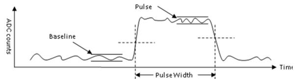
Figure 8: Edge detection of the beam pulse.
