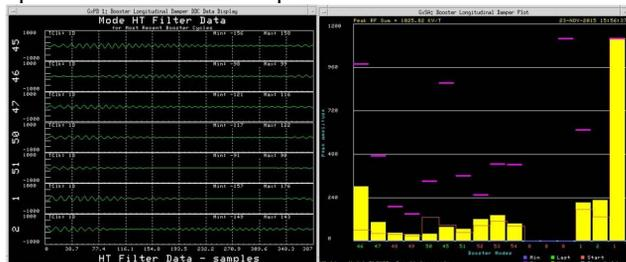
Figure 7: Damper diagnostics displays for mode error waveforms and mode peak amplitudes.
