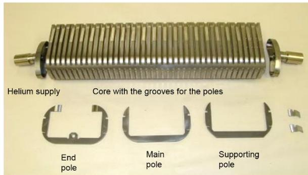
Figure 2: Core design modification.
