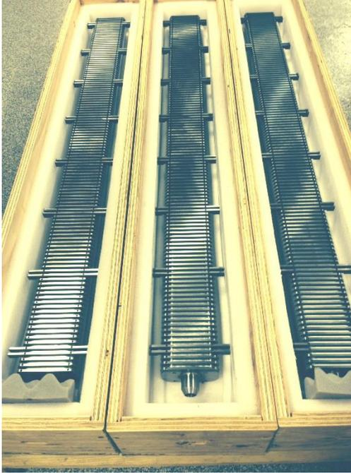
Figure 4: 1.5-meter-long cores prepared for shipment.
