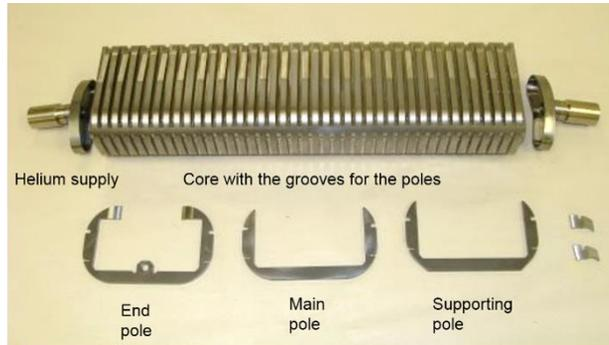
Figure 2: Core design modification.
