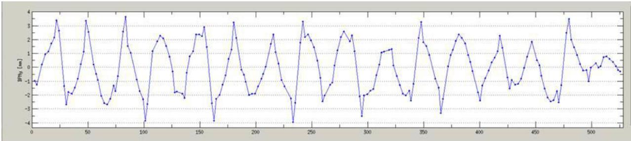
Figure 7 : Vertical closed orbit with all vertical correctors set to zero in the 3 GeV ring.
