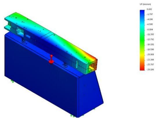
Figure 5 : FEA of gravity sag(U1), colour scale goes from 0 $\mu$ m(blue) to -28 $\mu$ m(red).
