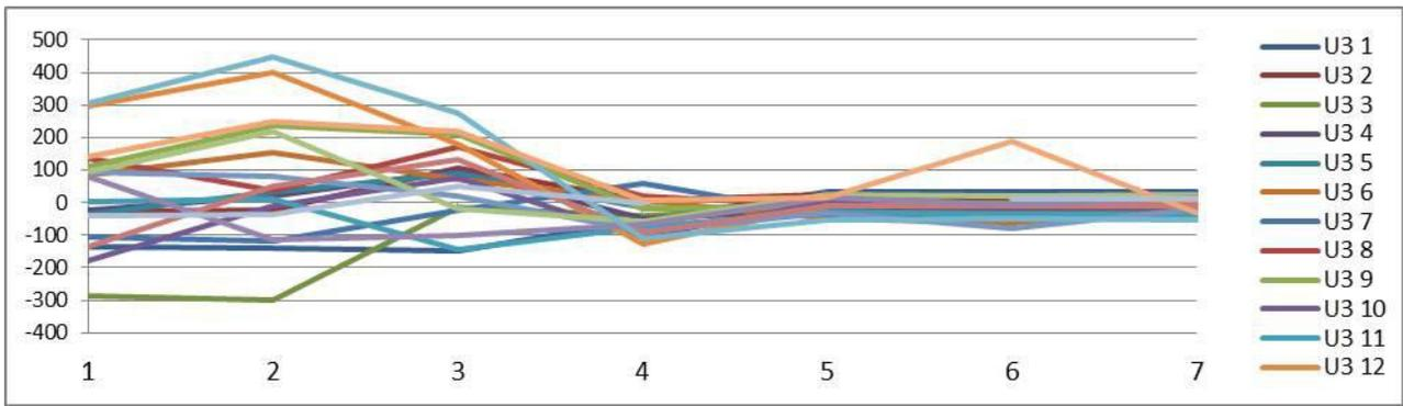
Figure 6: Straightness in microns of U3 magnets during the different stages in the process.
