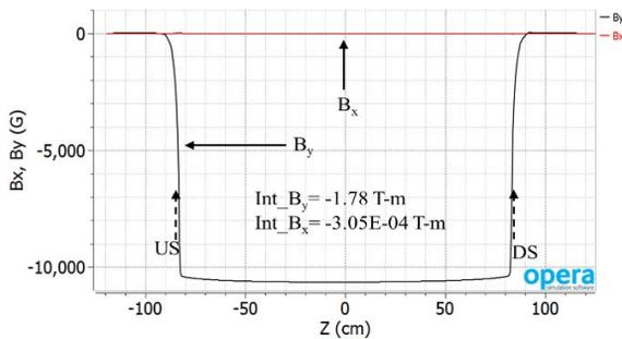
Figure 5:  $B_x$  and  $B_y$  fields along the injected beam trajectory. The red curve shows the  $B_x$  field and the black curve shows the  $B_y$  field.
