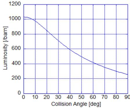
Figure 3: Luminosity dependence on colliding angle.
