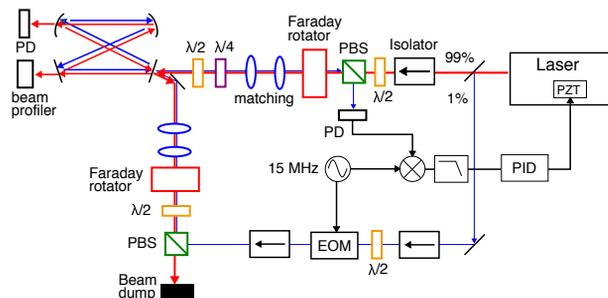
Figure 2: Setup of the optical cavity system.
