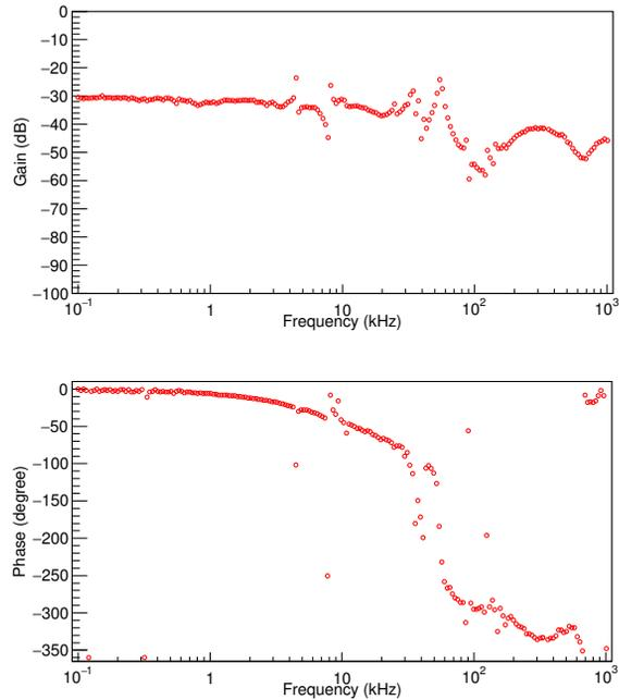
Figure 4: The measured frequency response of the piezo actuator.
