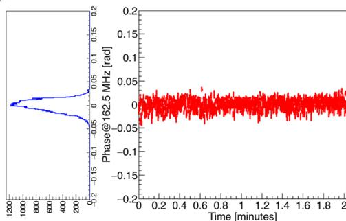
Figure 6: Stability of the laser phase in phase locking feedback.
