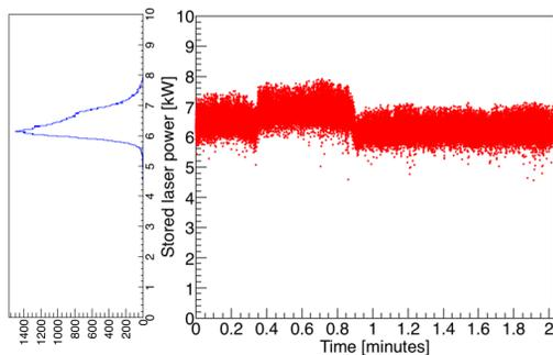
Figure 5: Stability of the stored laser power in the optical cavity.
