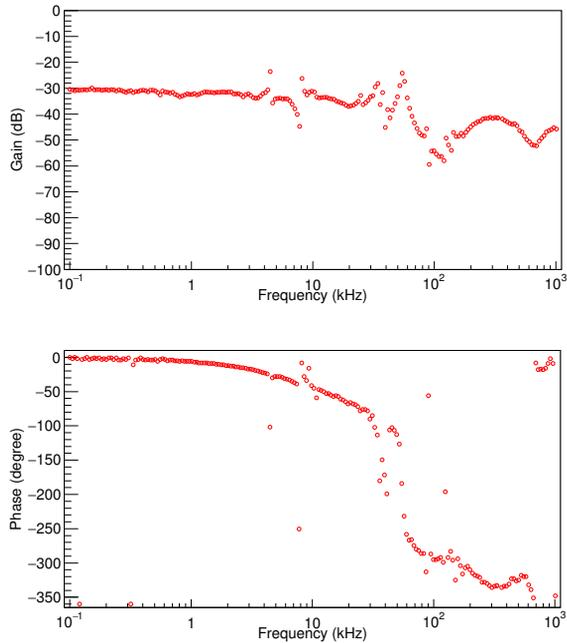
Figure 4: The measured frequency response of the piezo actuator.
