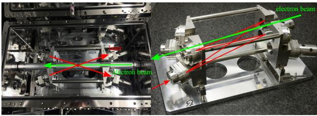
Figure 1: The optical cavity structure.
