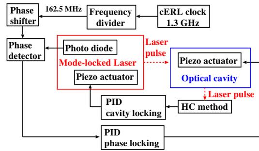
Figure 3: Block diagram of the feedback system.
