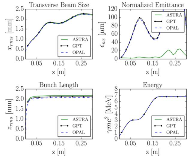
Figure 2: Beam envelopes in the gun.
