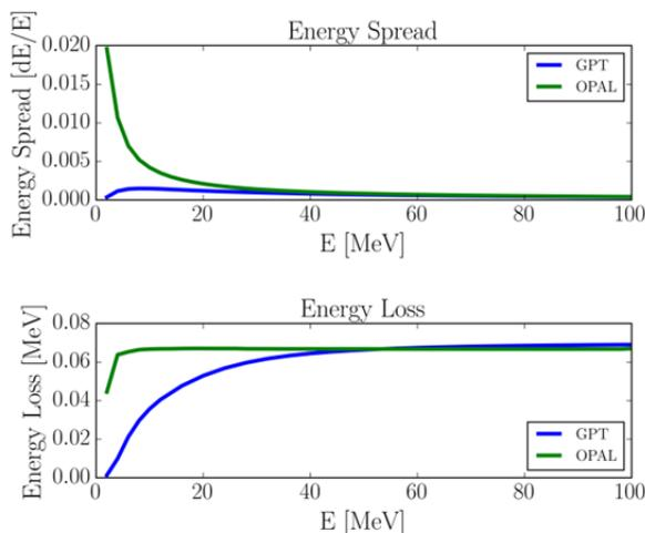
Figure 4: Energy spread and loss due to CSR.
