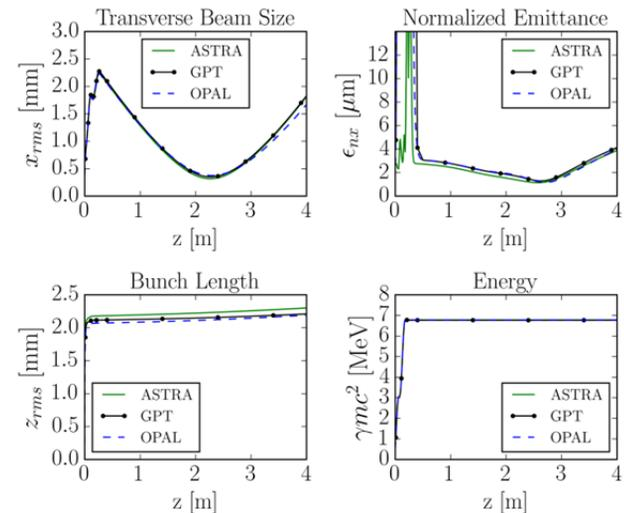
Figure 3: Beam envelopes in drift.
