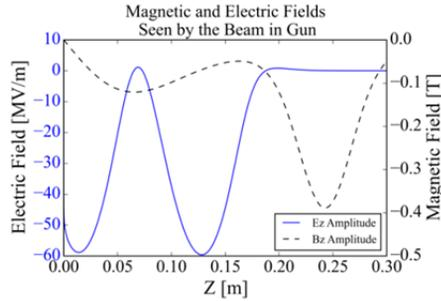
Figure 1: Magnet and electric fields in the gun.
