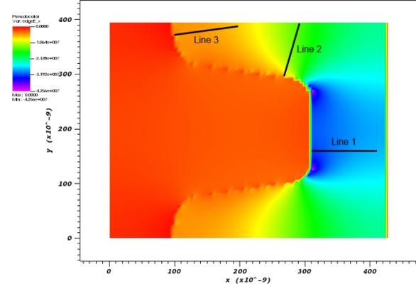
Figure 3: Longitudinal electric field from VSim's ES solver for the case of a single ridge rough surface confirms the strongest field enhancement is close to the tips of the ridge. The lines shown are normal to the ridge surface at the corresponding locations. The ES potential is calculated along such normals at positions where electrons attempt to cross the surface in order to calculate emission probabilities.
