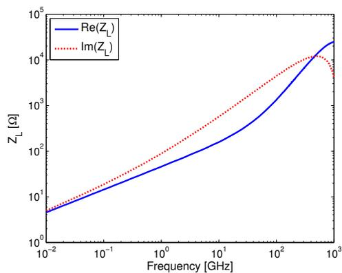
Figure 2: ALS-U total RW longitudinal impedance.
