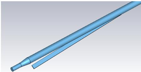
Figure 6: 3D models used for CST impedance simulations of the ALS-U x-ray egress.
