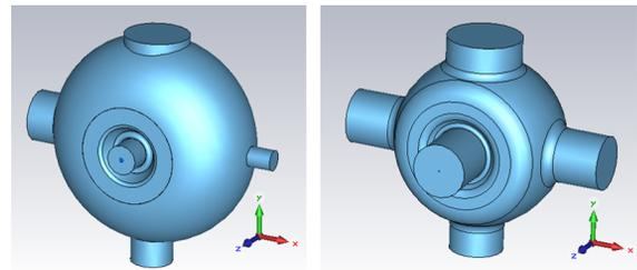
Figure 4: 3D models used for CST impedance simulations of the main cavity (left) and harmonic cavity (right).
