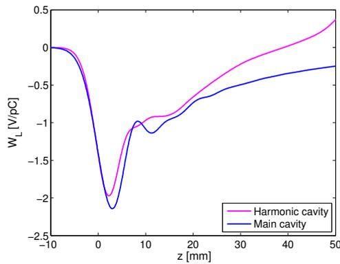
Figure 5: Wake functions of the main and harmonic cavities, calculated with CST Particle studio with a bunch length of 2 mm and wavelength of 500 mm and 150 mm, respectively.
