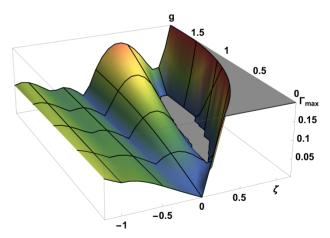
Figure 4: Growth rate of the most unstable mode for the Gaussian bunch with the resistive wall wake as a function of the head-tail phase and gain of resistive flat bunch-by-bunch damper. Gray color shows the "Lake of Stability".
