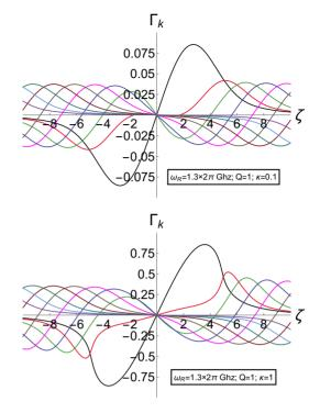
Figure 3: Coherent growth rates for the parabolic bunch with the wake function corresponding to CERN SPS impedance (broad-band resonator  $\omega_{\rm R} = 1.3 \times 2 \pi \,\rm{GHz}$ ) as functions of the head-tail phase. Top and bottom figures show different intensities.
