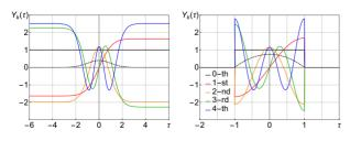
Figure 1: First five SSC harmonics  $Y_k(\tau)$  for Gaussian (left) and Hoffman-Pedersen (right) longitudinal distribution functions. Dashed black line shows line density of a bunch.
