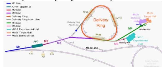
Figure 1: Layout of the Fermilab Muon Campus showing the beamlines for the Muon g-2 Experiment and Mu2e Experiment.
