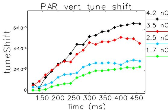
Figure 2: PAR vertical tune shift along the cycle.
