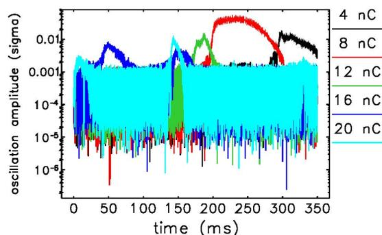
Figure 5: Simulated PAR vertical oscillation at high charge.
