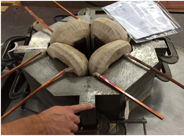
Figure 7: Production photo of one of the nine quadrupole magnets being manufactured by Stangenens. The quadrupole magnets are capable of creating 11 T/m field gradients over 24.8 cm effective length.
