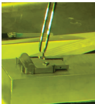
Figure 2: Half-shell of Mo target holder with irradiated Mo target disks. Disks are being extracted for processing.
