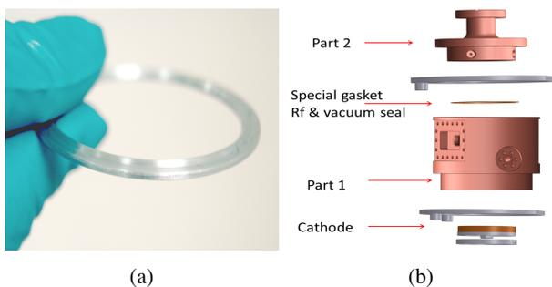
Figure 8: (a)  $2\frac{3}{4}$ " Aluminum gasket. (b) Clamping components.
