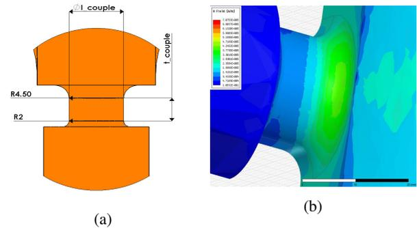
Figure 5: (a) Coupling port geometry. (b)  $H_{surface}$  map.
