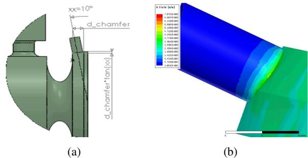
Figure 6: (a) Laser ports geometry. (b)  $H_{surface}$  map.
