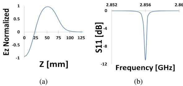
Figure 2: (a)  $E_z$  vs.  $z$  (b) S11 coefficient at resonance frequency,  $f_\pi$ .
