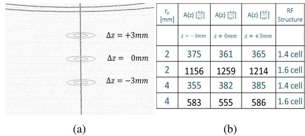
Figure 4: (a) Geometry of quadrupole moment measurement. (b) Quadrupole moment comparison table.
