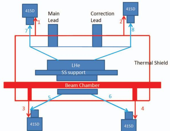
Figure 2: Cooling schematic of HSCU cryostat.
