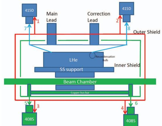
Figure 1: Cooling schematic of the planar SCU Cryostat.
