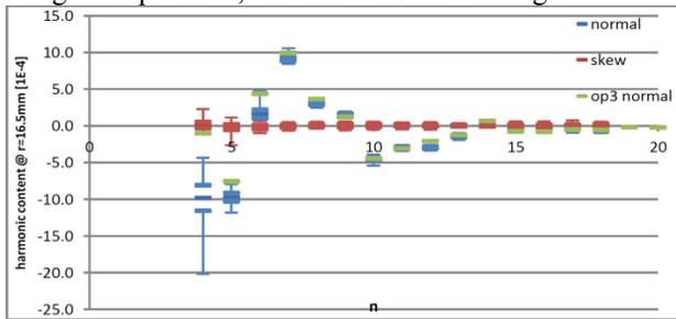
Figure 4: harmonic content higher order terms, boxplot of rotating coil measurement data for 48 pcs SQFo at nominal current, together with Opera-3d values [6].
