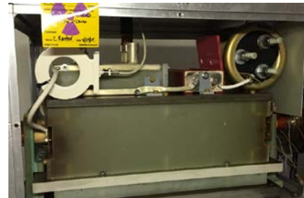
Figure 1: Photo showing free-wheeling diode added to stretch the abort kicker pulse.
