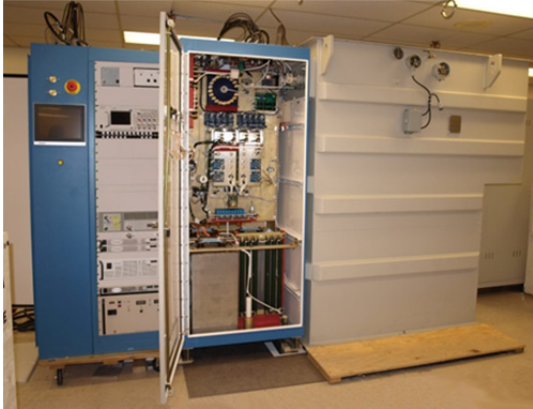
Figure 1: DTI's prototype solid-state ESS-class klystron modulator, developed under a DOE SBIR grant.
