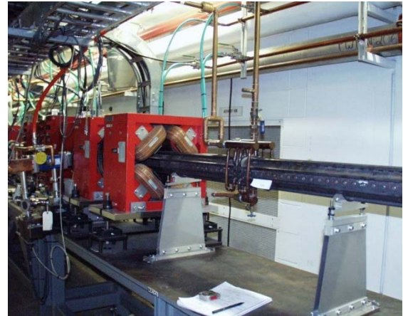
Figure 1: Original Linac structure located in the APS with quad magnets and rigid water lines.
