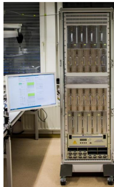
Figure 1: 100 kW 352 MHz pulsed SSPA prototype.
