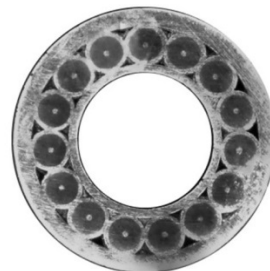
Figure 1: Cross-section of cable in conduit design.
