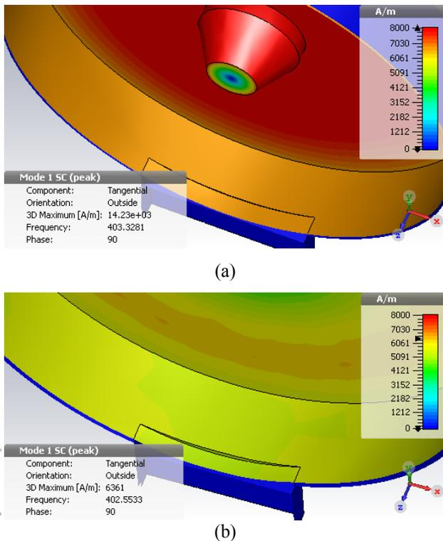
Figure 1: Surface current density distributions found with eigenmode simulation in (a) reentrant pillbox cavity (D: 17.88”) and (b) simple pillbox cavity (D: 22.44”). Surface curvature mismatches between test cavities and a waveguide iris coupler (D: 17.109” for SNS DTL1, 2).
