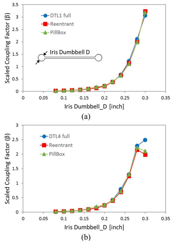
Figure 2: Comparison of scaled coupling factors of iris couplers with test cavities for (a) DTL1 and (b) DTL4.
