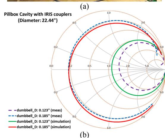
Figure 3: (a) Low power bench measurement setup with the cold model of a single-cell test cavity with waveguide iris couplers, (b) comparison of couplings of two couplers with simulated results.
