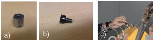
Figure 8: From left to right, a) fiducial fixtures, b)  $\frac{1}{4}$ " shank pin nest, and c)  $\frac{1}{2}$ " SMR.
