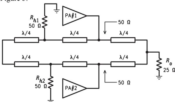
Figure 5: Two-input Gysel combiner.
