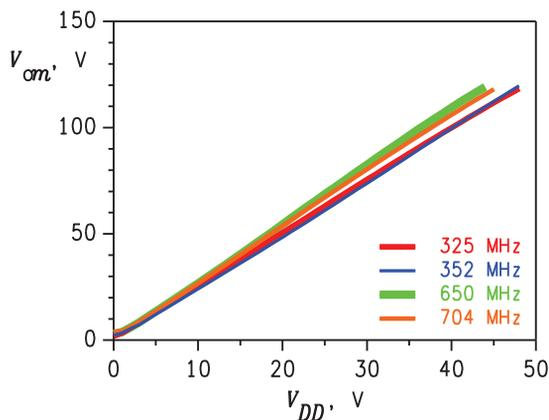
Figure 4: Amplitude linearity of final amplifiers.
