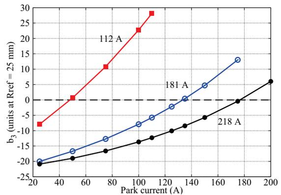
Figure 6:  $b_3$  as a function of park current at three operation currents: 112, 181, and 218 A. An offset of  $-3.67$  units for the geometric and saturation effect based on the measurements from the spare D96 magnet was applied to the calculation.  $R_{\text{ref}} = 25$  mm.
