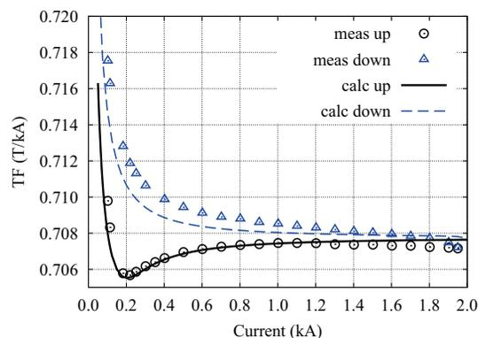
Figure 2: Comparison between the measured and calculated transfer function. Circle: measured data during the up ramp after precycles. Triangle: measured down ramp. Black line: calculated up ramp. Blue line: calculated down ramp.
