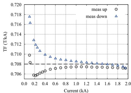
Figure 1: The measured dipole transfer function from the “DC loop” measurements. Circle: measured data during the up ramp after precycles. Triangle: measured data during the down ramp. The dashed line at 0.708 T/kA is the geometric value of the transfer function.
