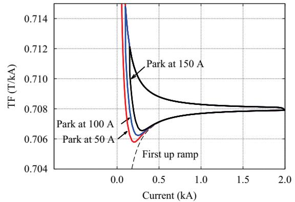
Figure 5: Impact of park currents on the dipole transfer function. Three park currents are calculated: 50, 100, and 150 A.
