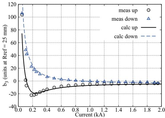
Figure 3: Comparison between the measured and calculated  $b_3$ .  $R_{\text{ref}} = 25$  mm. Circle: measured data during the up ramp after precycles. Triangle: measured down ramp. Black line: calculated up ramp. Blue dashed line: calculated down ramp.
