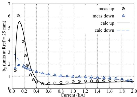
Figure 4: Comparison between the measured and calculated  $b_5$ .  $R_{\text{ref}} = 25$  mm.
