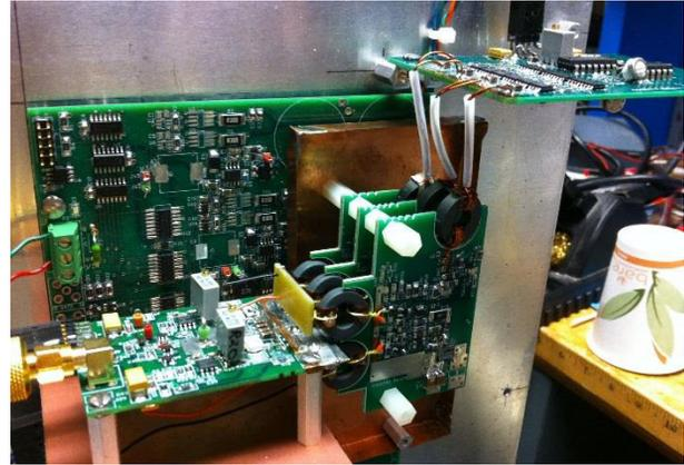
Figure 4: Switch assembly. Trigger generator board is on the lower left, the 3-FET switch is center-right and AC power delivery PCB is upper-right. The load is not shown in this photo.
