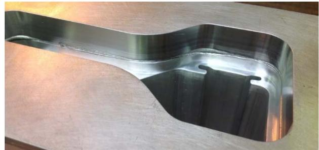
Figure 4: Automated 2 mm thick aluminium profile weld.
