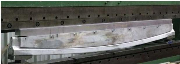
Figure 2: Bending of an L-bend chamber extrusion.
