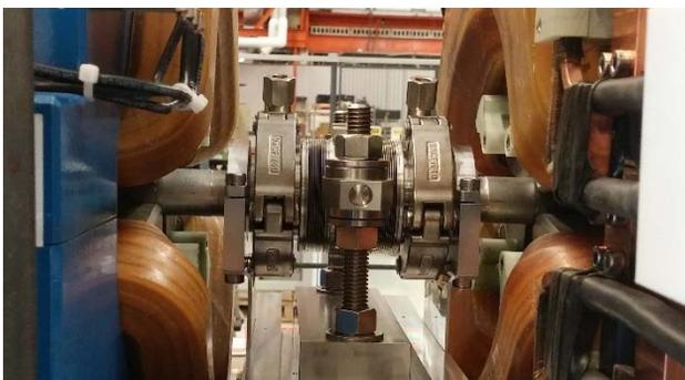
Figure 3: Mock-up BPM in an integrated test assembly.
