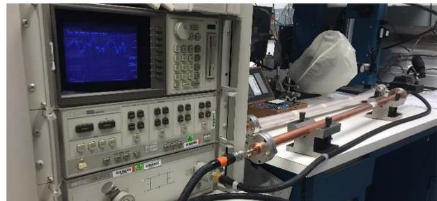
Figure 6: Network analyzer measurements on a copper vacuum chamber prior to NEG coating.
