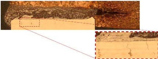
Figure 5: Stress fracturing in electron beam welds.
