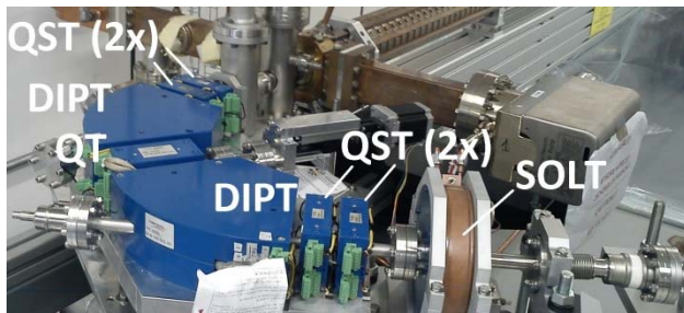
Figure 3: energy filter magnets between thermionic gun and first accelerator structure at Solaris 2014.
