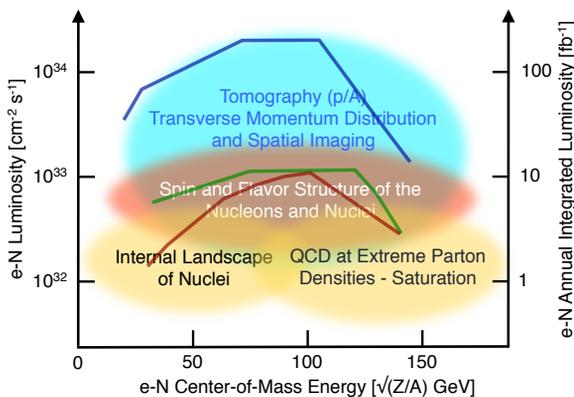
Figure 1: Luminosity vs CME of various considered eRHIC designs overlapped with eRHIC physics areas. Green curve- Initial ERL-Ring design, red curve - Initial Ring-Ring design, Blue curve- Ultimate ERL-Ring design.
