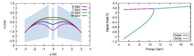
Figure 4: The split arc dipole layout with electron orbits at different energies (left plot) and the outer and inner section magnetic field vs the beam energy (right plot).
