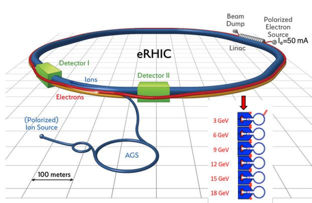
Figure 2: The ERL-Ring design option layout.
