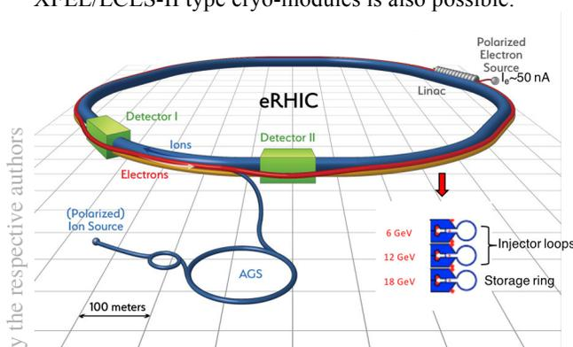
Figure 3: The Ring-Ring design option layout.
