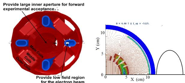
Figure 5: IR magnet design developed for eRHIC. “Sweet spot” design (left plot), and the active shielding design (right plot).
