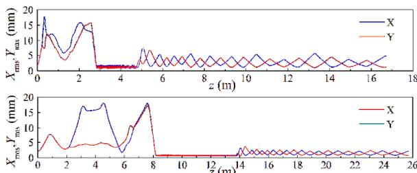
Figure 9: RMS beam envelopes along the front-end: deuterium ion beam (top), lead ion beam (bottom).
