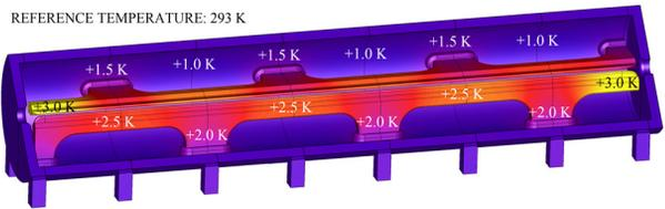
Figure 6: Temperature change steady state distribution over the Light Ion RFQ resonator.
