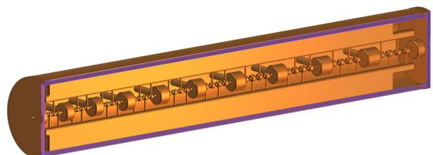
Figure 8: 3D model of the IH-1 section with FODO focusing lattice.
