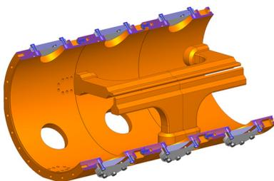
Figure 5: Tank segments and vanes of the 4-vane resonator with magnetic coupling windows for Light Ion RFQ.
