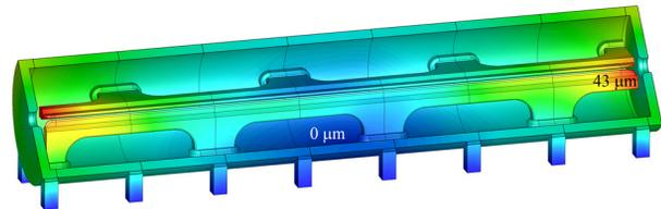
Figure 7: Deformation of the resonator, including effects of gravity, atmospheric pressure and heating.
