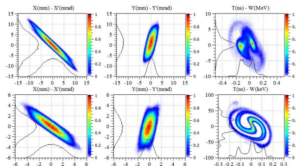
Figure 10: Output phase-space plots of the deuterium ion beam (top) and lead ion beam (bottom).
