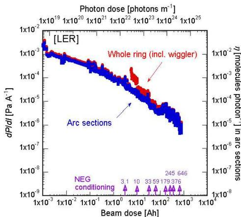
Figure 2: Pressure rise and expected photon stimulated gas desorption rate as a function of beam dose in the LER .
