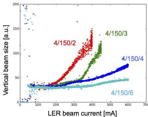
Figure 5: Beam-size blowup (vertical) in the LER.
