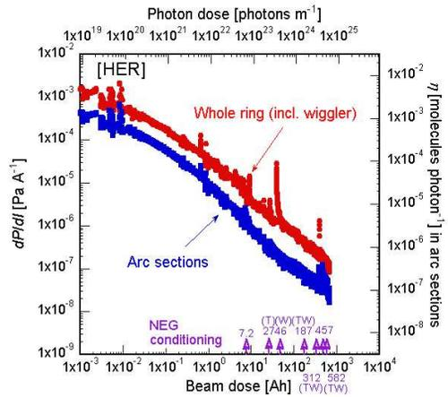
Figure 3: Pressure rise and expected photon stimulated gas desorption rate as a function of beam dose in the HER.
