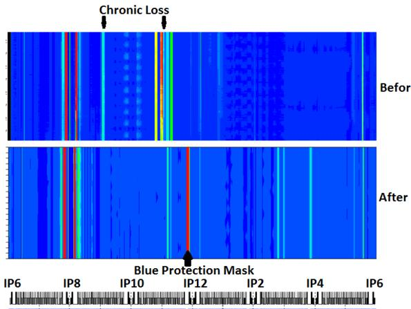
Figure 2: The chronic beam loss nearby protection bumps area before and after modification.
