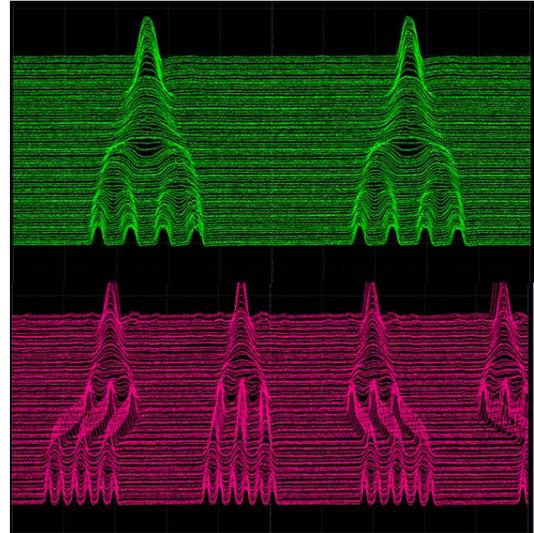
Figure 1: Merge scheme in the AGS for 8→4→2 (top) and 12→6→2 (bottom).
