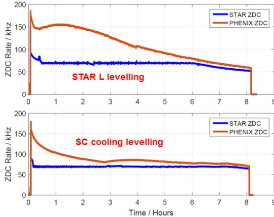
Figure 4: STAR luminosity levelling with 70 kHz ZDC rate (top); SC cooling levelling was used for higher integrated luminosity for STAR.
